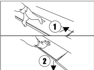
5• Position the following strip end-to-end with the preceding one, inclining it at an angle of around 30 degrees, while fitting it against the horizontal tongue ( ① verrouillage longitudinal).
