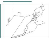
4. Use the off-cut of the first row to start the second one, ensuring that this is at least twice the width of the strip itself for aesthetic reasons. Adjust the strip and click it into place having rotated it.
