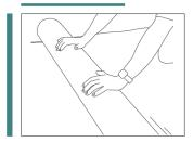
1. Roll out an insulating polythene underlay, such as ISOL 30, ensuring the subfloor is flat and dry. The panels are taped together side by side and should fit along the bottoms of the skirting boards.
