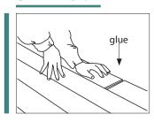
6• Cut the strips for the final row to the required width, including an expansion gap. Fit them together flat with a metal pull bar. Add a small amount of glue on each plank tongue widthwise, removing any excess glue. 24 hours after laying the floor, remove the wedges. Cover the expansion gap using suitable fittings such as skirting boards, radiator rings and threshold strips.
