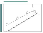
2• Start to lay the strips in a corner, facing the wall and moving from right to left. Position the tongue side of the strip against the wall, and cut the tongue off to allow for the expansion gap. Insert wedges in the expansion gap.
