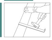
5. Cut the last row of strips to the required width, allowing for an expansion gap. Fix them into place flat with a metal pull bar. 24 hours after laying the floor, remove the wedges and cover the expansion joints using suitable fittings such as skirting boards, radiator rings and threshold strips.
