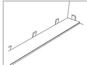
2• Start to lay the strips in a corner, facing the wall and moving from right to left. Position the tongue side of the strip against the wall, and cut the tongue off to allow for the expansion gap. Insert wedges in the expansion gap.
