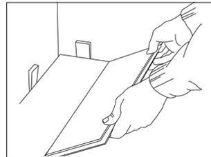
4• Use the off-cut of the first row to start the second one, ensuring that this is at least twice the width of the strip itself for aesthetic reasons. Adjust the strip and click it into place having rotated it.
