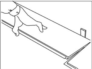
3• Add a small amount of glue on each plank tongue widthwise, removing any excess. Place the second strip at the end of the previous one. Continue like this for the first row, glueing each widthwise, but only on this row.
