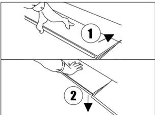
5• Position the following strip end-to-end with the preceding one, inclining it at an angle of around 30 degrees, while fitting it against the horizontal tongue ( **1** verrouillage longitudinal).
