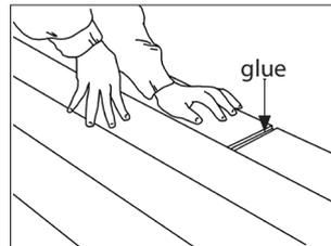
6• Cut the strips for the final row to the required width, including an expansion gap. Fit them together flat with a metal pull bar. Add a small amount of glue on each plank tongue widthwise, removing any excess glue. 24 hours after laying the floor, remove the wedges. Cover the expansion gap using suitable fittings such as skirting boards, radiator rings and threshold strips.
