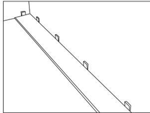
4• Place wedges around the sides to create an expansion gap.
