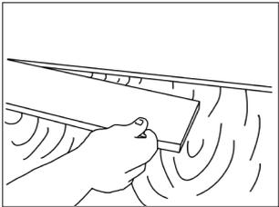
3• Place the flooring strip or panel into the glue and press down to ensure that it adheres properly.
